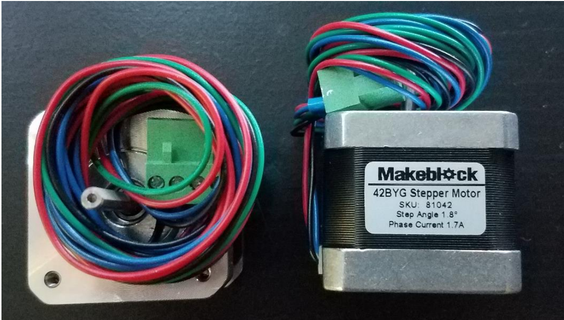
Figure 9: Makeblock Stepper Motors.
